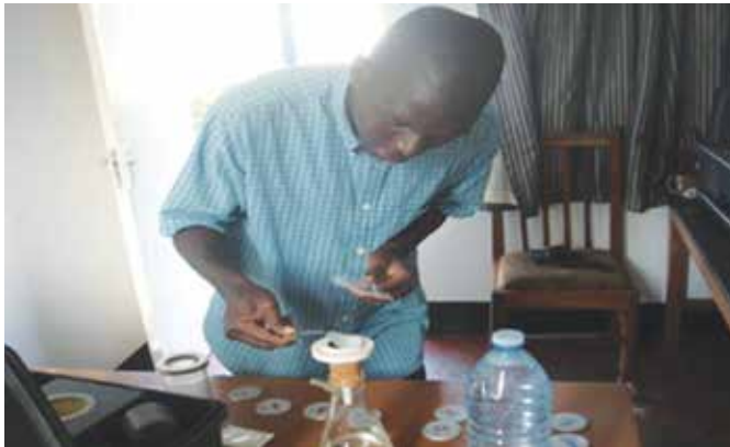
Figure 3: Placing a sterile-membrane filter on the apparatus
