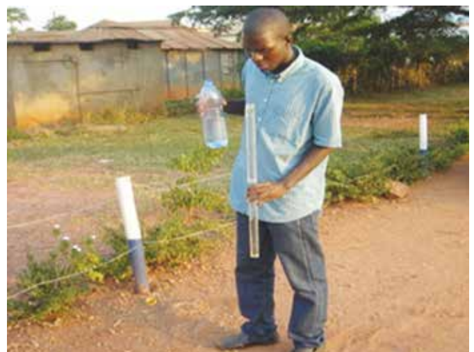
Figure 2: Measuring turbidity using a turbidity tube
